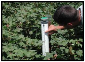
Fig. 1. Measuring potential ET in SDI management plots with an ET gauge.
